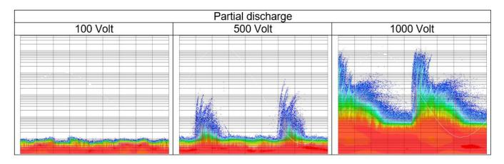
However, the discharge of a cavity can also lead to several discharge structures (fingers). This depends on the geometry, field distribution, permittivity and other factors. The cavity discharges take place at the greatest voltage change. The consequence of this partial discharge is a slow but
